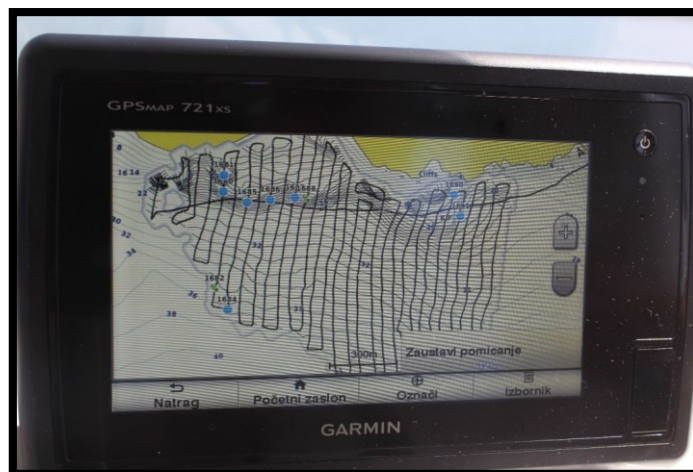
Picture 9. Created contour map for the northern end of the surveyed area.
