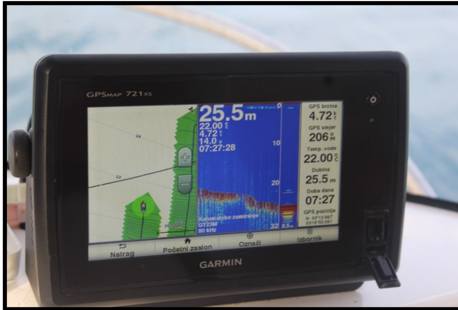
Picture 6a. Contour mapping along a single transect in the target area and in real time.
